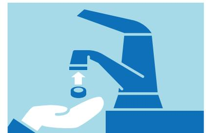
**6** Replace all point-of-use filters, including the filter in refrigerators. Clean and reinstall or replace aerator screens.
